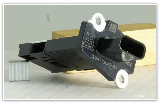
Mass airflow sensors can become contaminated from PCV vapor, a potting compound leak from the circuit board, unburned fuel, water – even a spider searching for a new home. Unfortunately, visual inspection usually won't reveal if contamination caused a sensor to fail; nor will it determine if a sensor still functions.
