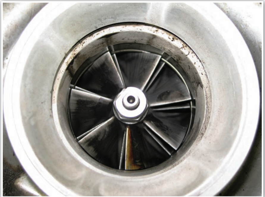
A Ford dealer diagnosed this turbocharger from an F350 6.0L engine as having bearing failure due to dirt ingestion. An oil analysis indicated silica content in the oil at 7ppm (extremely low) indicating no problems with the air filtration equipment. Upon inspection the shaft / impeller assembly rotated freely and was in good working order.
